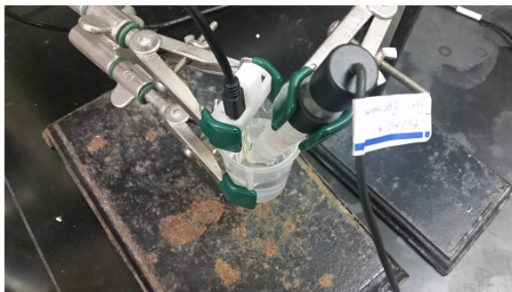
Figure S9: Electrochemical cell (top-view) used for LSV electrolyte switching experiments
